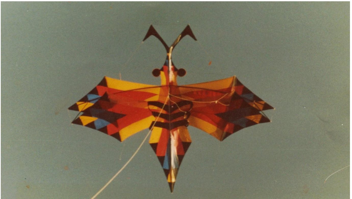
9m wingspan Dragonfly kite 1984, violent weaving reduced by moving the bridle point down.
