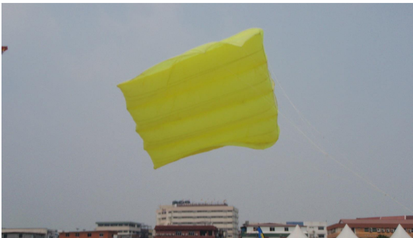
Ram air pilot kite leaning off because of rearward lateral area disposition. Sarawak, August 2009
