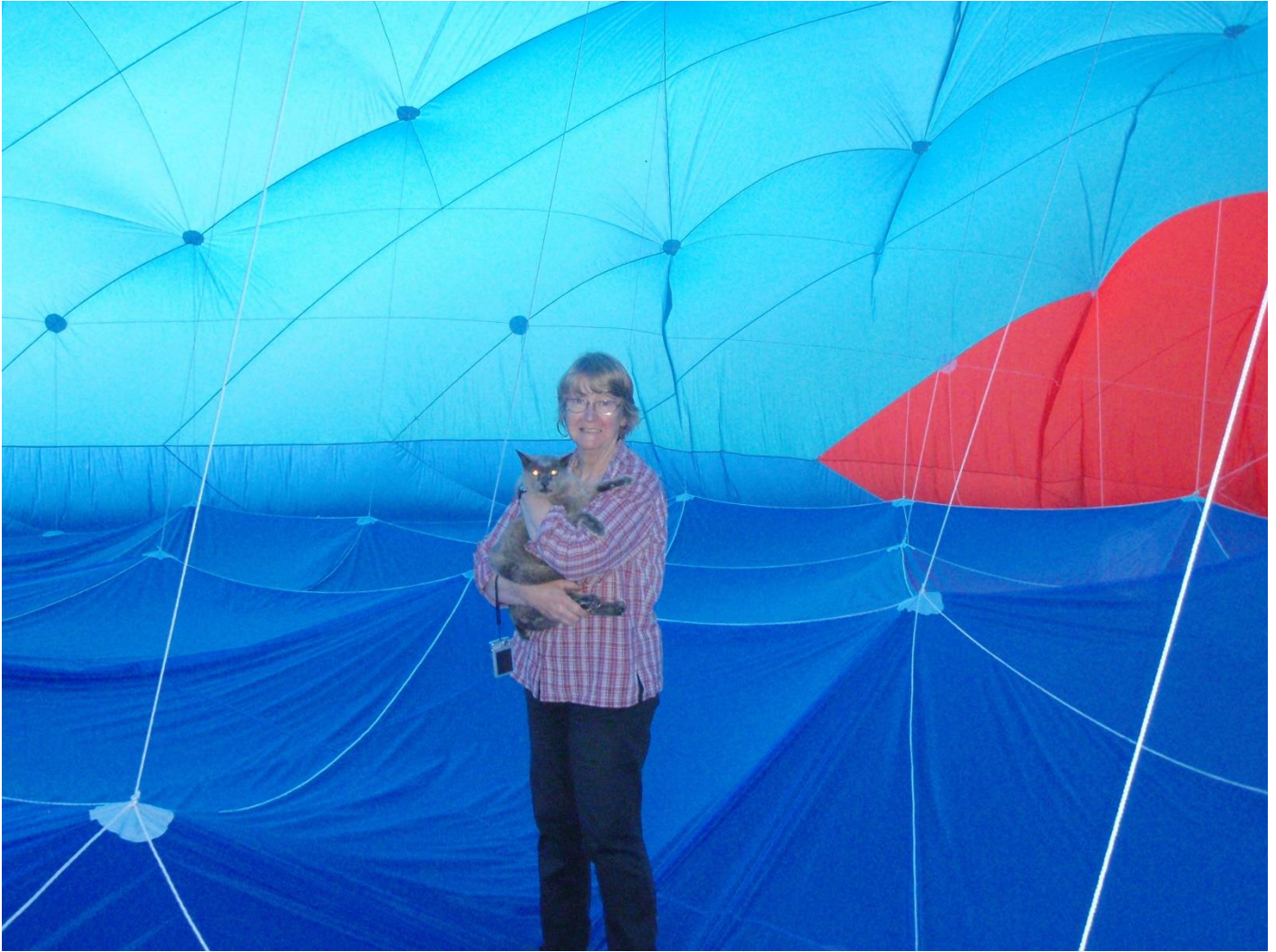
Inside the 1250 sq. m ‘Pearl’ mega ray showing use of thru cords instead of ribs- and Elwyn and Tory
