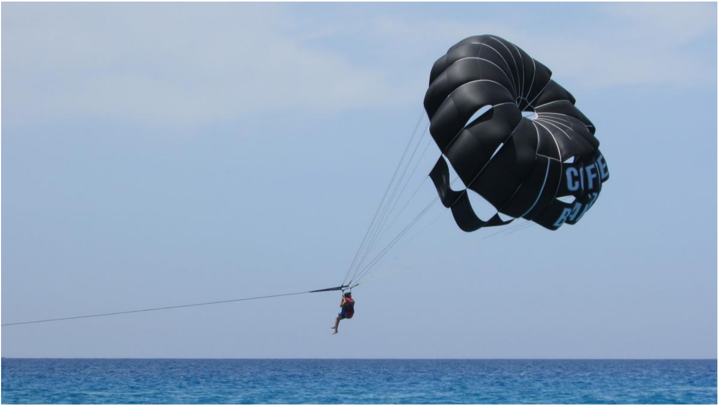
Towed parasail: Righting moment is very high, weaving can't establish- but swinging can.
