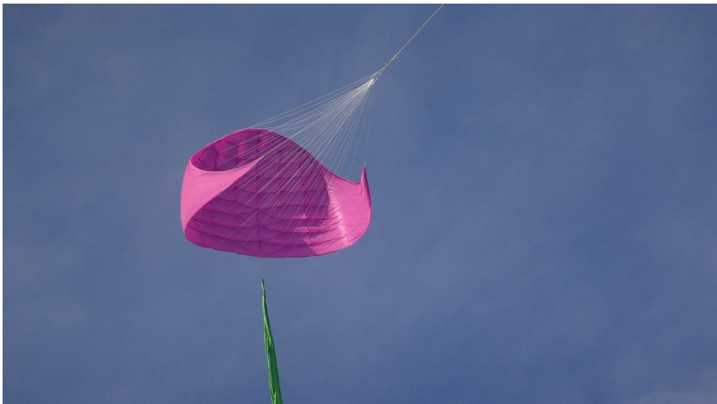
Underneath view of 3sq.m SSSL Serpent head with rear flares- dived over, wouldn't fly at all.
