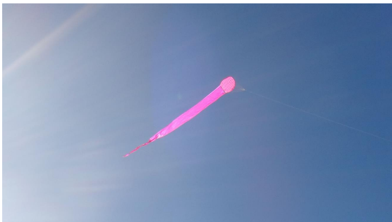
20m SSSL Serpent: just 0.1 sq. m increase in lateral area dealt to weaving instability.
