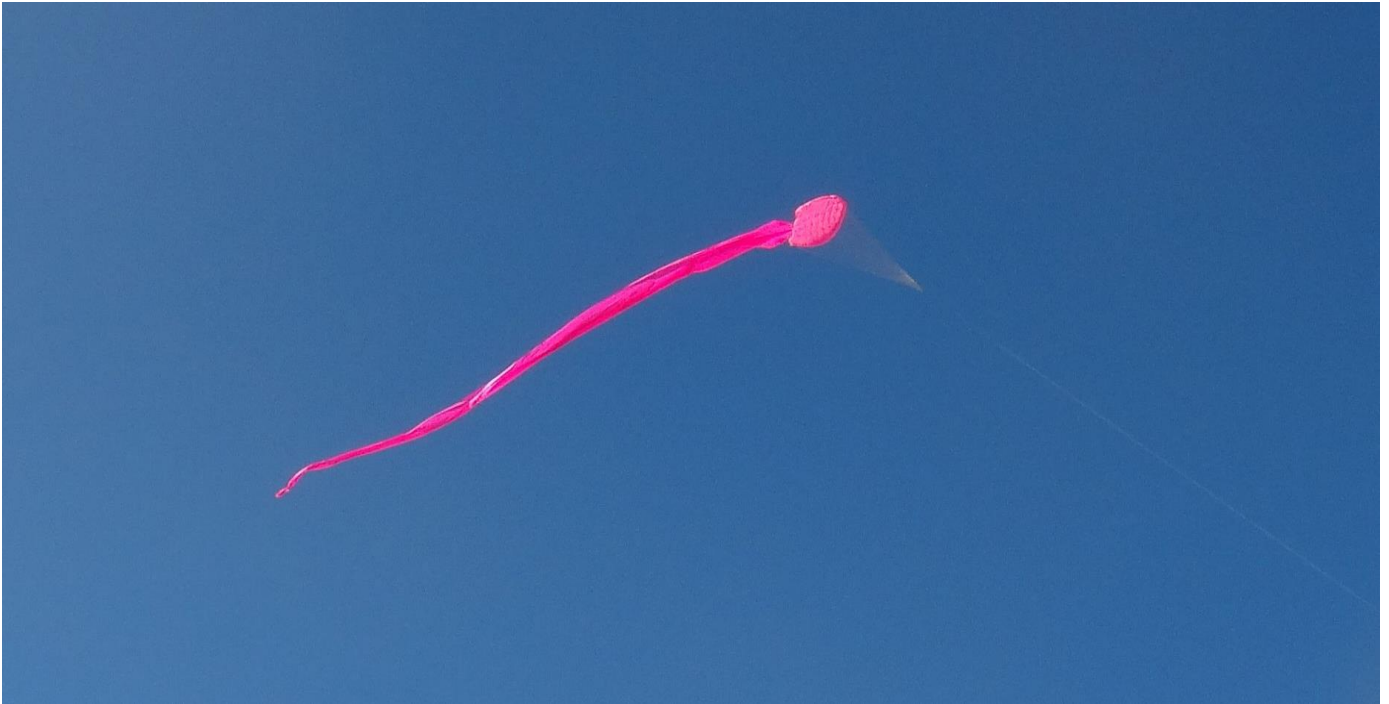
20m Serpent with tail attached half width- significantly higher weaving instability onset.
